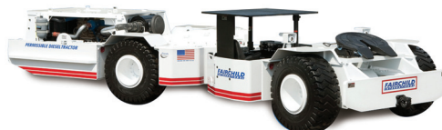
35C-WHPDT Workhorse Permissible Diesel Tractor
